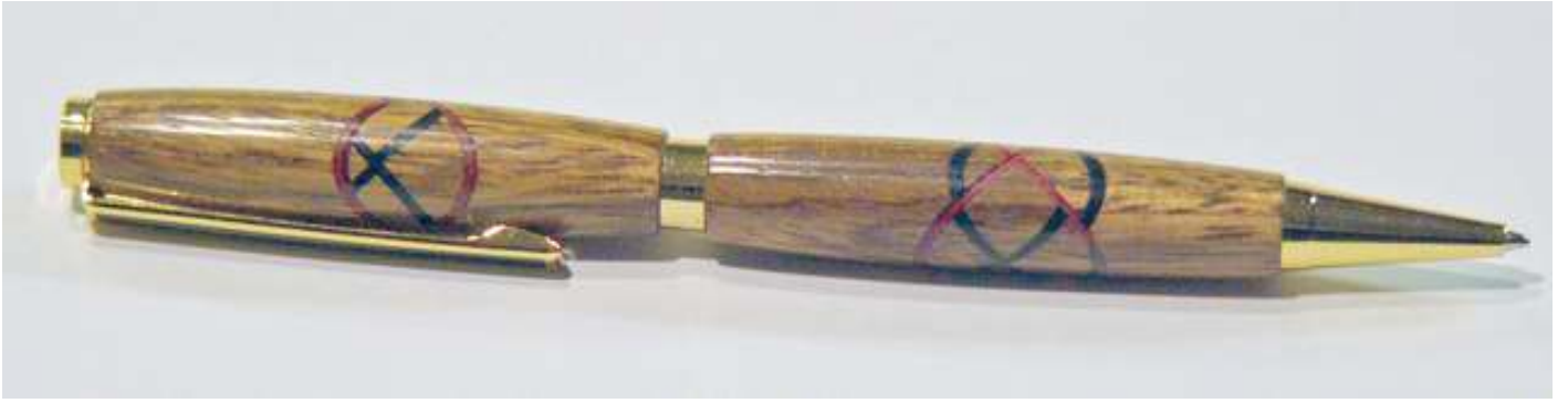
The finished pen with black and red dyed veneer segments
