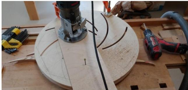
The photo to the left shows the routing process about half-way through, and the one below shows the same level of completion without the trammel base and router in place.
