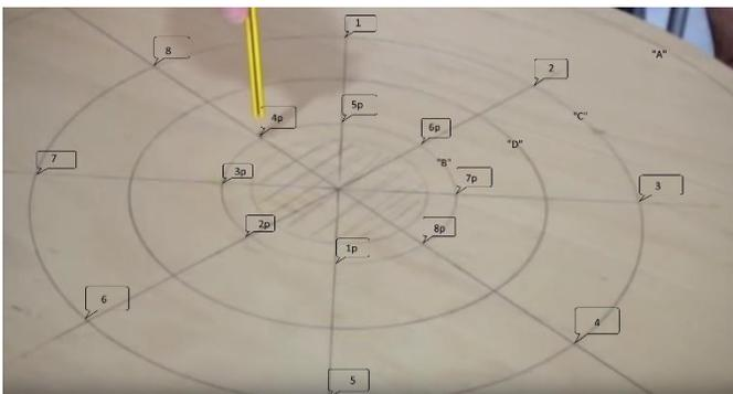
Example: place the compass pivot point at location "1", and the pencil at location "1p". Moving the pencil to the left, draw an arc beginning at "1p", and ending on circle "A". Repeat for each of the points on circle "C".
