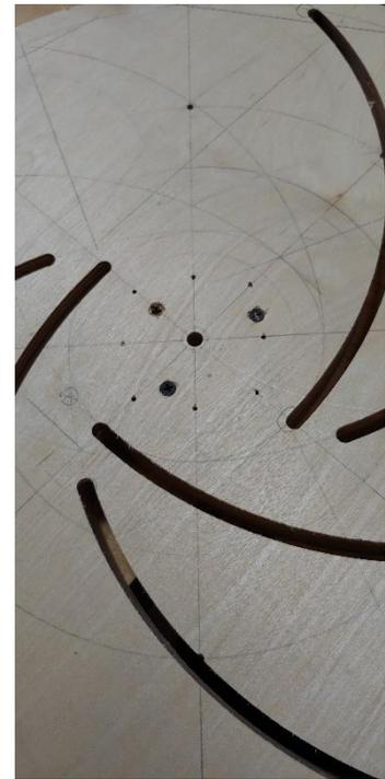
To complete the chuck after routing out the arcs, do the following steps. First, drill a series of finger holes along the outer edge. You can see these in the photo below. Drill them all the way through both disks, sand them, and if you like, round over the edges with a palm router and a 1/8” roundover bit. Here’s a close-up:
