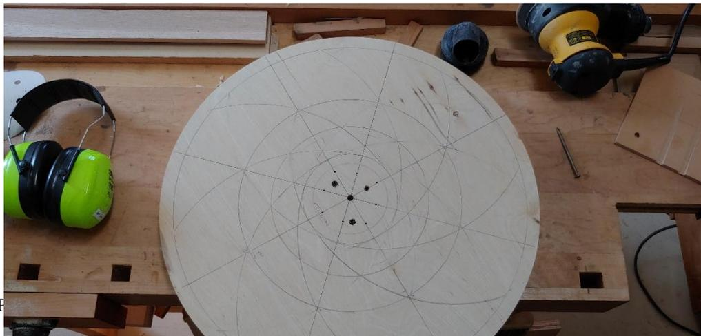
Next step is to make a trammel base for your router, if you haven't already made one for other projects. A trammel base is just a fixture that lets you route an accurate circle. In this case, the diameter of the arc you'll cut is the same as the distance from points "1" and "1p". You want to be accurate when you lay out this trammel base and when you make it. Here is what I made for this project:
