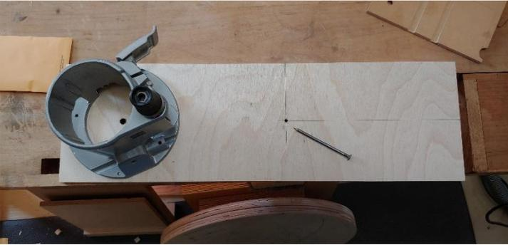
Here is the trammel base in position on the disk, at the beginning of the waste removal process. Note that I raised the disks up off my workbench with some scrap, because the router bit is eventually going to
