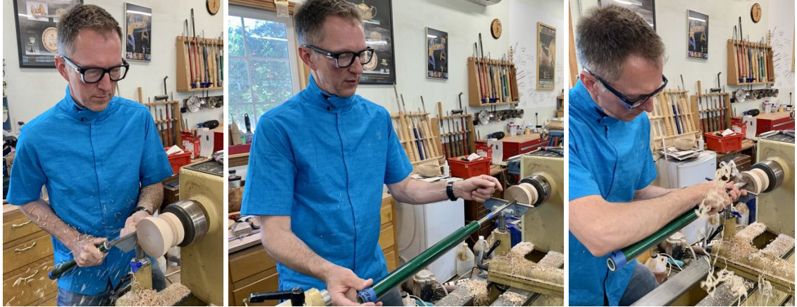
*Forearm control of scraper; diamond hone; the setting*
