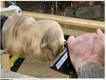
\*Then he went back to the straight scraper, then to an Elsworth with an offset bit and on to another with a HSS bit longer cutter focusing on getting the top ½ to the final thickness before going deeper.
