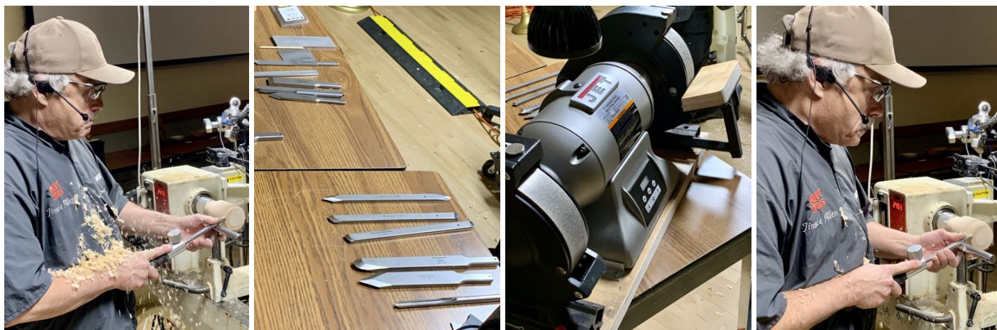
Above: Jimmie often uses his tools unhandled for light, finishing cuts.
