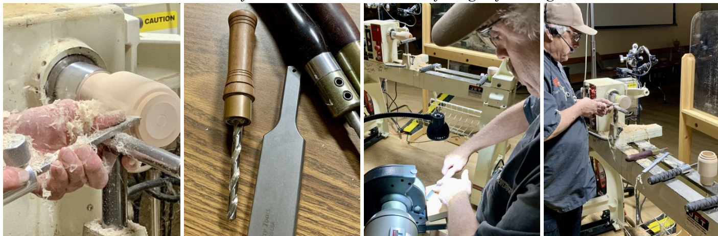
Above: Making the tenon for the lid, his hand drill, the 3 second sharpening pass.
