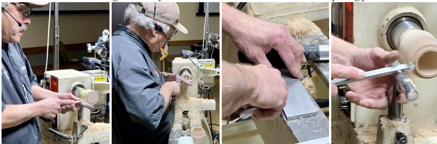
Above: Quick touch up on a diamond stone, close up of his finger wrapped around the post of the tool rest, his preferred method for control.
