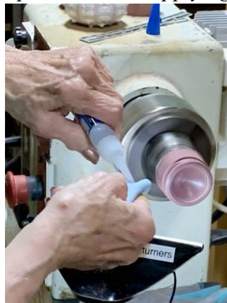
Above: foam filled shell, parting sections for finial/box top/base/foot; measuring for box size; turning box Below: color coded sandpaper and tools; applying CA finish; turning lid; drilling hole in lid for finial
