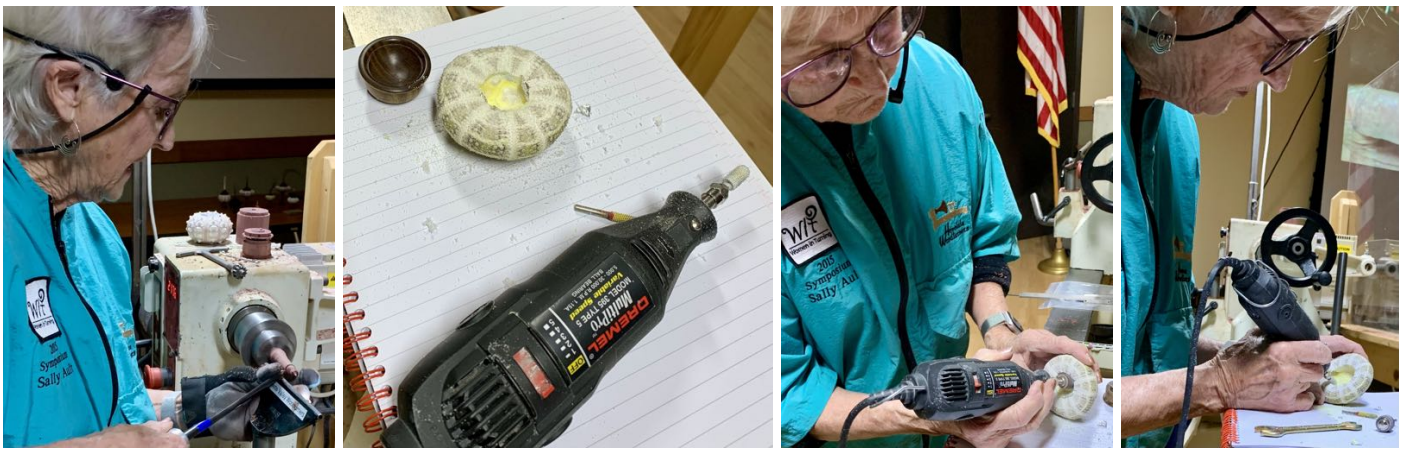
Above: turning finial; cutting hole for box with Kutzal (sp?) burr; squaring up sides of hole with sanding drum Below: lots of refinement of hole; tools (sewing ruler at bottom); box in hand; Sally was totally willing to continue conversation after demo!
