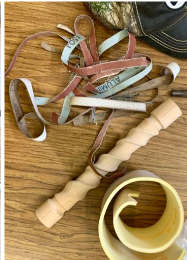
Above: in-progress examples of "mark outs" and spirals with different numbers of bines and pitches; rasps, zesters and sanding sticks; sandpaper for "flossing"; small rasps and burs Below: examples of open twists, different pitches, and zesters
