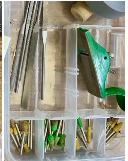
Above: in-progress examples of "mark outs" and spirals with different numbers of bines and pitches; rasps, zesters and sanding sticks; sandpaper for "flossing"; small rasps and burs Below: examples of open twists, different pitches, and zesters
