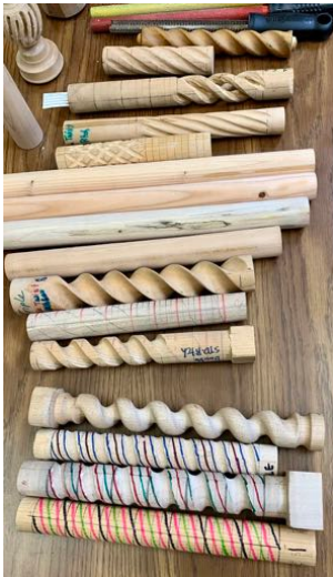
Above: in-progress examples of "mark outs" and spirals with different numbers of bines and pitches; rasps, zesters and sanding sticks; sandpaper for "flossing"; small rasps and burs Below: examples of open twists, different pitches, and zesters
