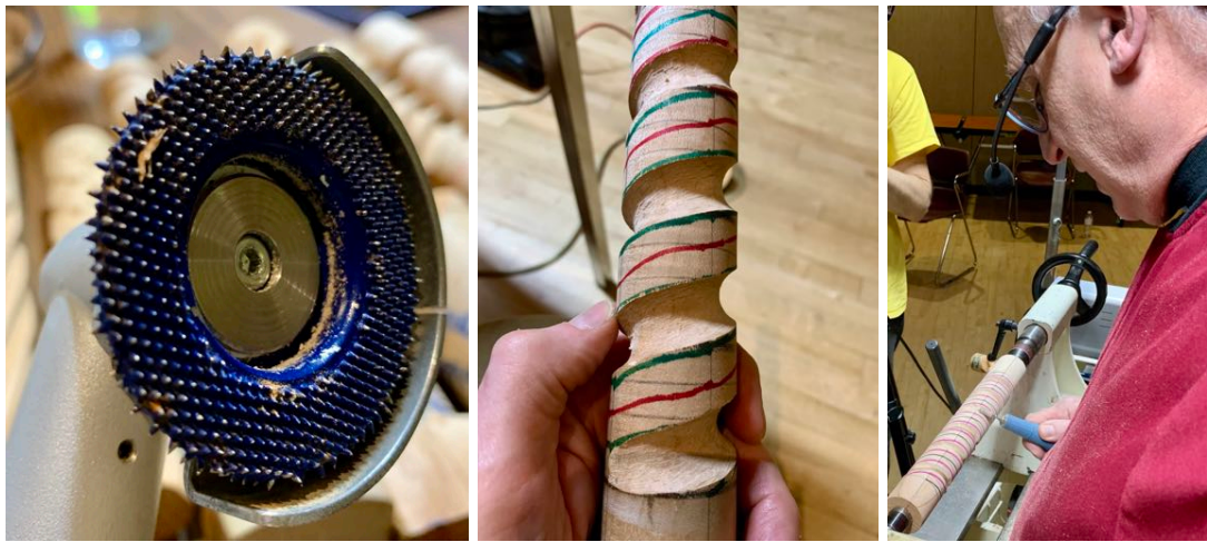
Above: large burr carver, valleys in progress, micro-carver with burr
