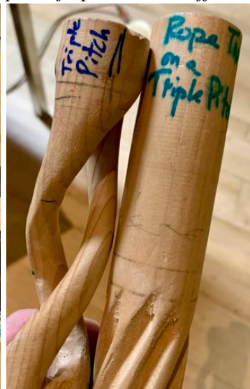
Above: in-progress examples of "mark outs" and spirals with different numbers of bines and pitches; rasps, zesters and sanding sticks; sandpaper for "flossing"; small rasps and burs Below: examples of open twists, different pitches, and zesters
