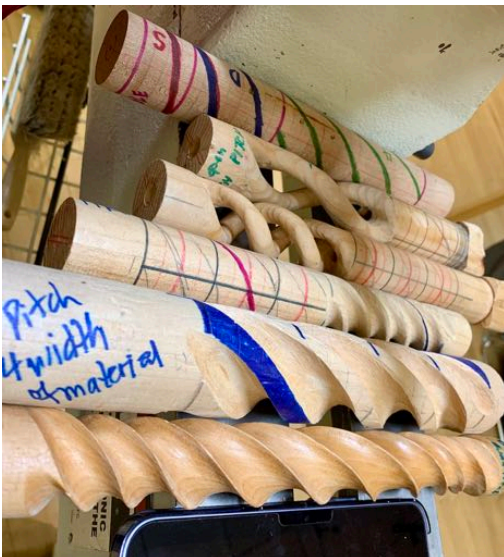
Above: in-progress examples of "mark outs" and spirals with different numbers of bines and pitches; rasps, zesters and sanding sticks; sandpaper for "flossing"; small rasps and burs Below: examples of open twists, different pitches, and zesters
