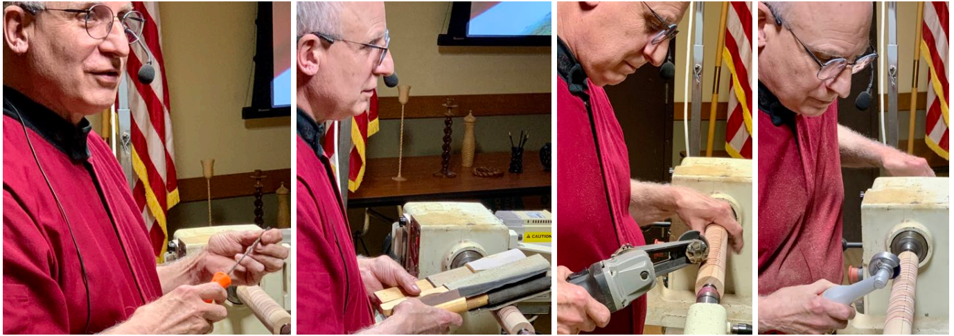
Below: drill/rasp Terry likes for open twist spiral making, sandpapers sticks, two styles of power carvers
