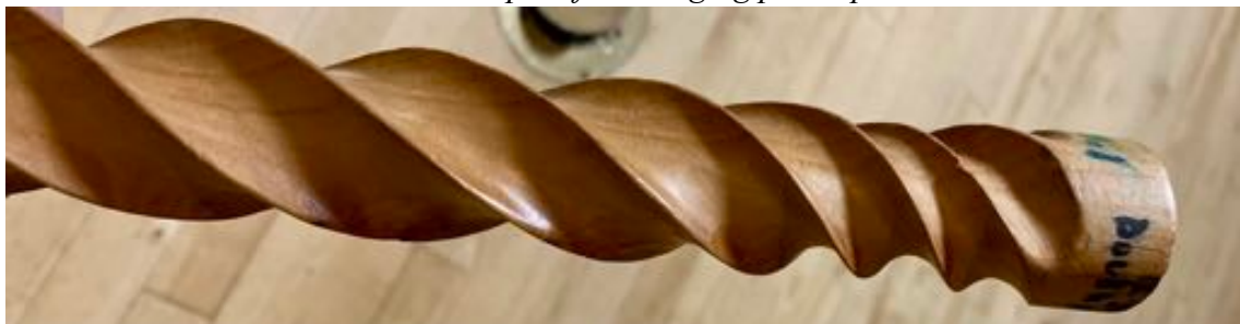
Below: example of a changing pitch spiral
