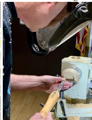
Above: parting the lid/base, turning top of lid, inside of lid with tenon ready for brass insert Below: top of lid, testing insert in base recess, hollowing base
