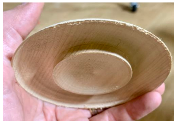
Above: parting the lid/base, turning top of lid, inside of lid with tenon ready for brass insert Below: top of lid, testing insert in base recess, hollowing base
