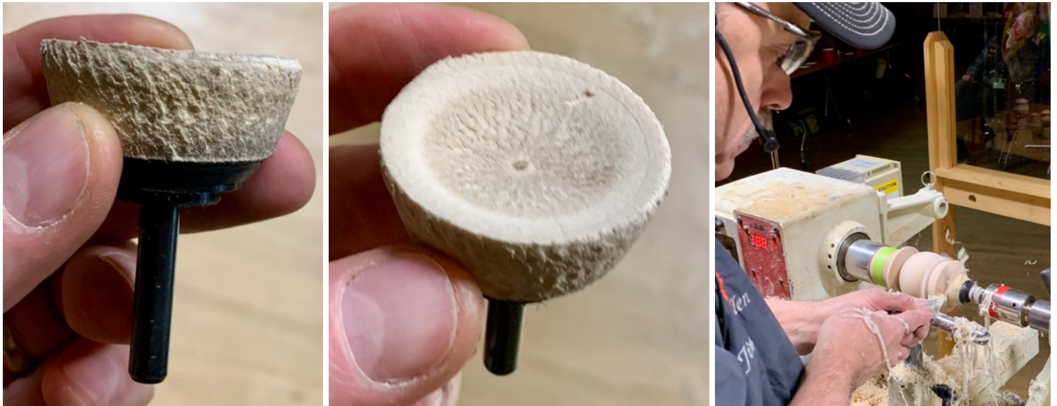
Below: Jimmie uses a spent sanding mandrel (hook and loop material gone) as a rotating jam chuck fitting it into a live center with a removable tip; refining the top
