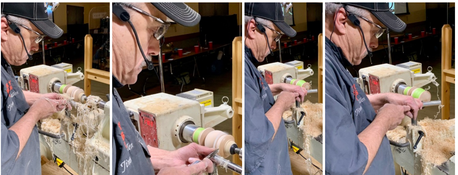
Above: refining, refining; to finalize top Jimmie added some tape to the joint for extra security-he used a spindle gouge for final cuts for final cuts
