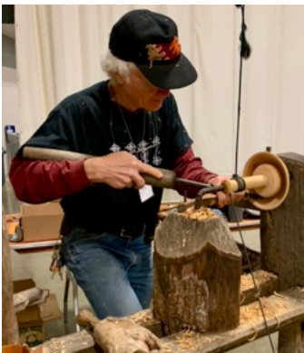
Below: Kiko with the strongest leg in turning. All his gouges are homemade and hook style.
