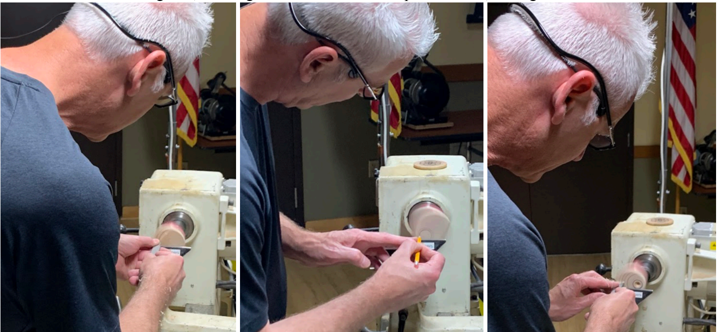
Below: cutting arcs, marking circle on other side for pendant hole, cutting arcs on backside
