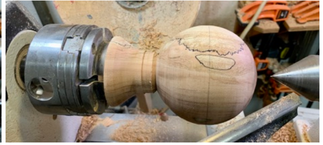
Left: My daughter Dana is a goldsmith in Corvallis and came to Elizabeth's demo. She made a mold for this ring with texturing inspired by the demo. Below: This is how I made a couple kuksa cups using the chuck to gain access to the complete sphere.
