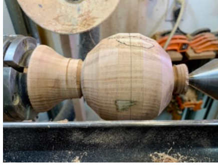
Left: My daughter Dana is a goldsmith in Corvallis and came to Elizabeth's demo. She made a mold for this ring with texturing inspired by the demo. Below: This is how I made a couple kuksa cups using the chuck to gain access to the complete sphere.
