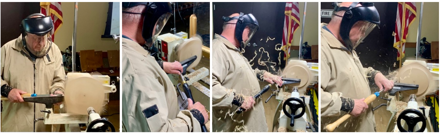
Above: Once reversed, he had to do a little truing and then he began the hollowing, again working from the corners in and leaving the bulk of the center mass.
