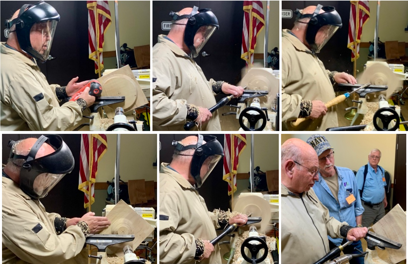
Above: Tom cuts to thickness moving in about 1" at a time to help with vibration.
