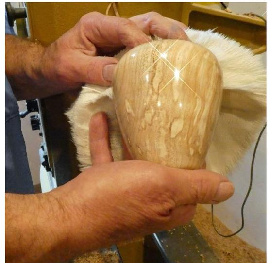
*Run the buffing wheel at about 1000 RPM. Hold the piece securely.*
